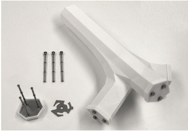
5 The metal detail components and the PLA molds © PSL.
