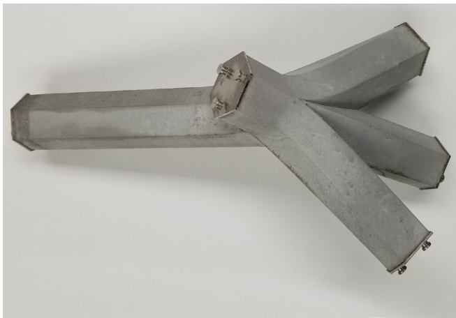
6 A spatial node with its steel connections after demolding © PSL.
